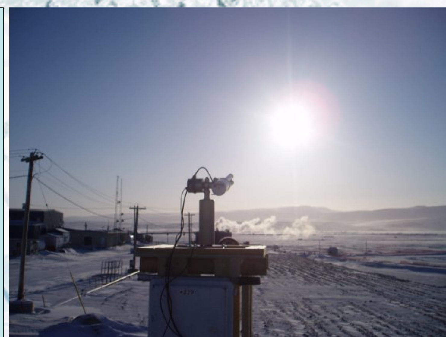
AEROCAN CIMEL Sunphotometer located at PEARL Eureka. AEROCAN is a subnet of AERONET
